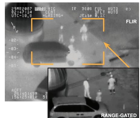
Range-Gated Imagery Compared to FLIR Imagery
